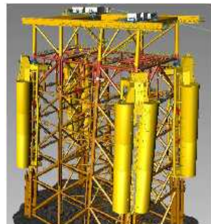
Figure 44: Refloat of jacket using added buoyancy tanks
