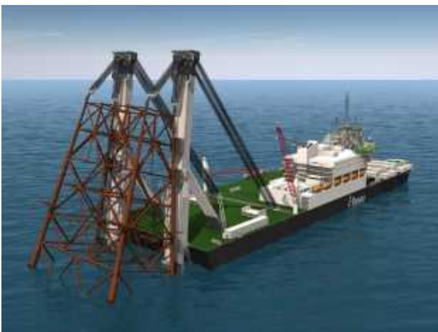
Figure 43: Jacket Removal Using a Single Lift Vessel
